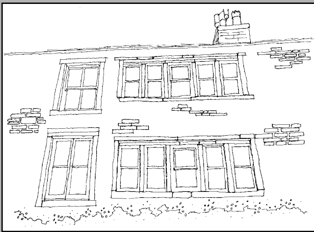
Fig 2 : Sash window (upper left) and stone mullion weaver window (upper right)
